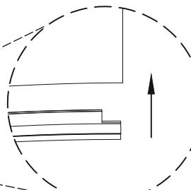
Vid behov: After installation remove protective tape and clean aluminum profile with petroleum or ethanol (or similar).
